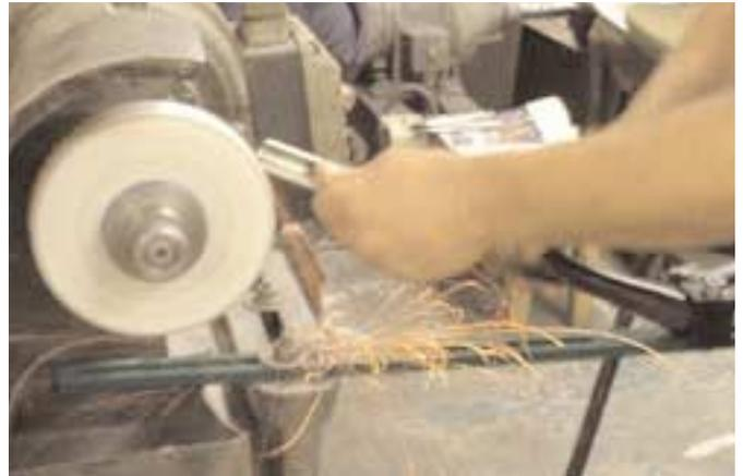
**The jig could not be simpler to use**, yet the results are totally consistent accuracy. We all know the necessity of not just using the correct tools, but in having them sharpened so as to give maximum performance. This jig is the answer to bowl gouges with extended wings.
